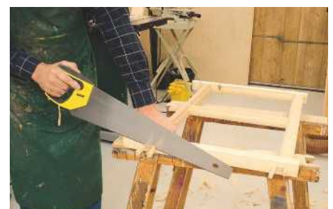
▲ Pic.23 The sashes are sanded, the horns and wedges are cleaned off level and the rebate formed in the bottom rail
